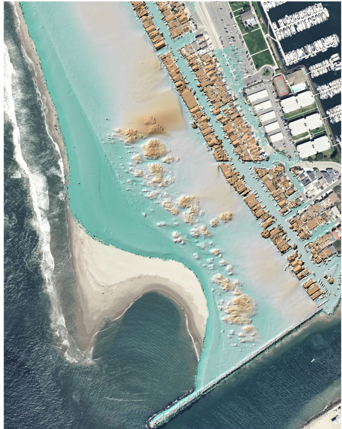
Example Digital Terrain Model (DTM) from 2023. This model will be used to support evaluation of dune growth and stabilization through time
